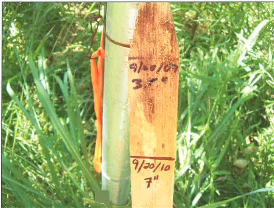
BF 2 Crest Gage on the mainstem of Davis Branch (Year 2). (EMH&T, 9/20/10)
