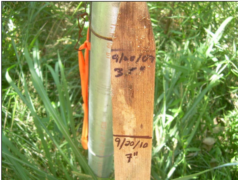
BF 2 Crest Gage on the mainstem of Davis Branch (Year 2). (EMH&T, 9/20/10)
