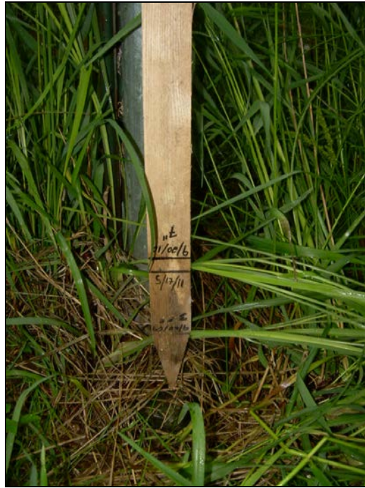
BF 3 Crest Gage on the mainstem of Davis Branch (Year 3). (EMH&T, 9/14/11)
