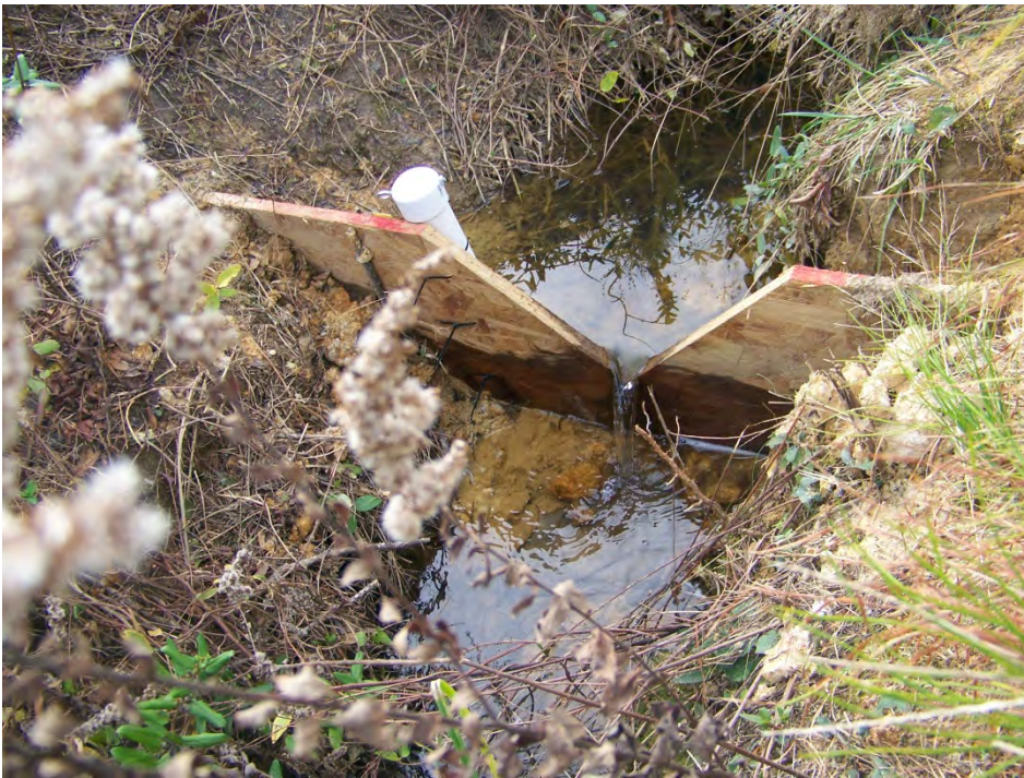
Streamflow monitoring weir on Southwest Branch
