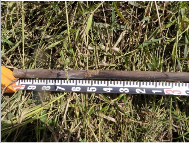
Crest Gauge – 3.54 feet (Storm event occurred on October 1, 2010)
