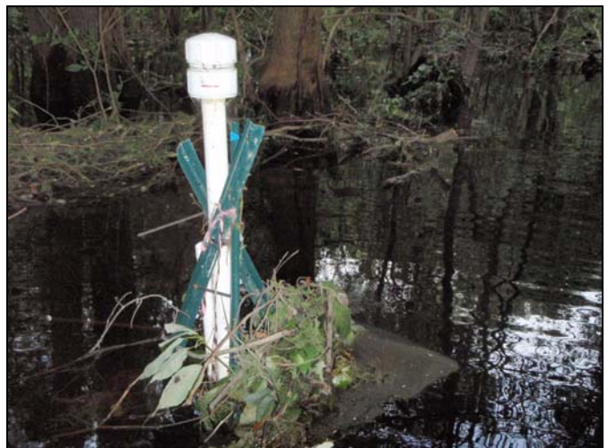
Flood gauge 1 with wrack from Hurricane Irene (Storm event occurred in August 27, 2011)
