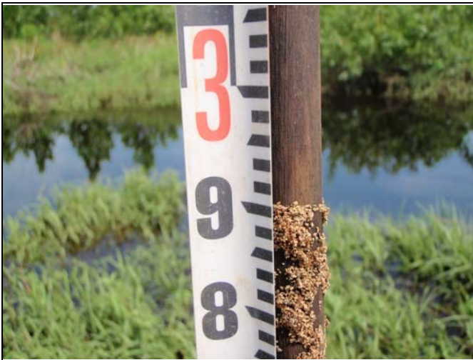
Crest Gauge – 2.90 feet, following Hurricane Irene (Storm event occurred on August 27, 2011)
