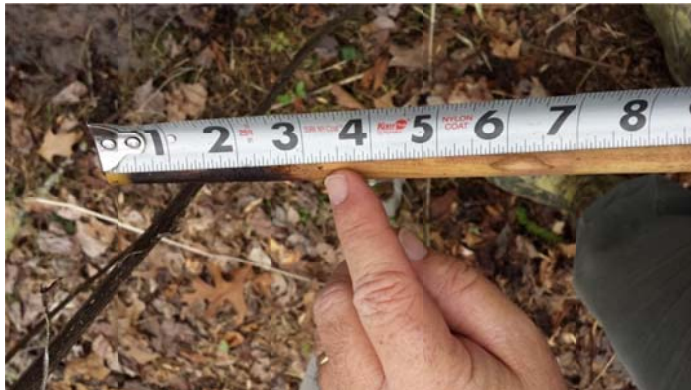
Photo of staff and cork at 3.25 in above bankfull, from UT2 crest gauge.
