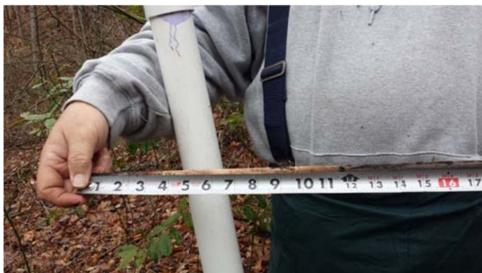
Photo of staff and cork at 4 in above bankfull, from UT6 crest gauge.
