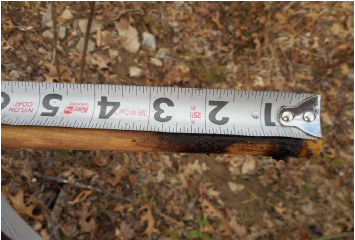
Photo of staff and cork at 2.25 inches above bankfull, from UT2 crest gauge.
