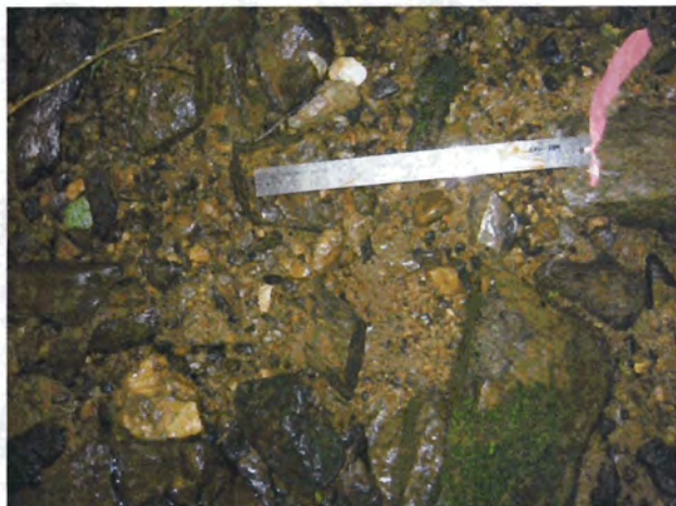
Photograph 19. Example of bed material along Cross Section #1, Reach A, UT Cabin Branch. Ruler is 15 inches long. (5/25/05)
