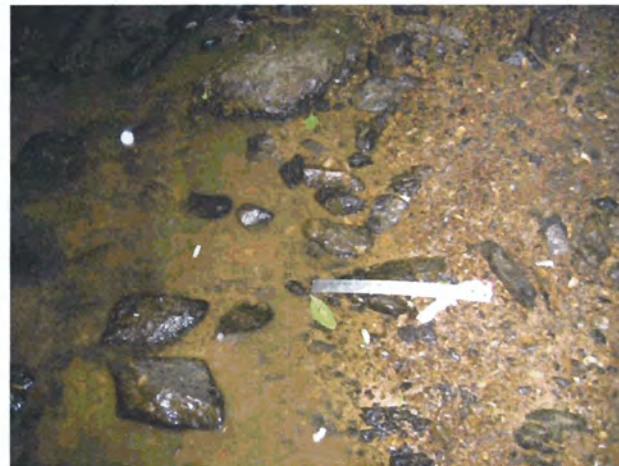
Photograph 20. Example of bed material along Cross Section #1, Reach A, UT Cabin Branch. Ruler is 15 inches long. (5/25/05)
