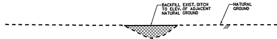
TYPICAL DITCH - SECTION DITCHES 1, 2, 3, 5, 7, 16, AND 17 NOT TO SCALE
