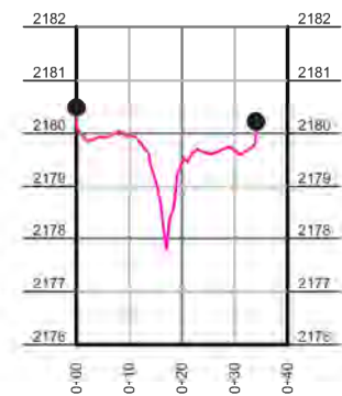
CROSS-SECTION #1-HARRELL CREEK HORIZONTAL SCALE: 1" = 40' VERTICAL SCALE: 1" = 4'
