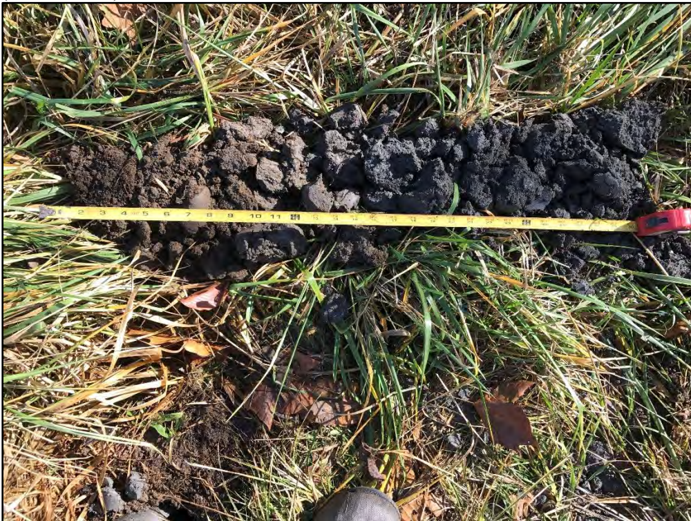
2. Soil Meets A5- Stratified Layers, A12-Thick Dark Surface, and F6-Redox Dark Surface (Profile # 104).
