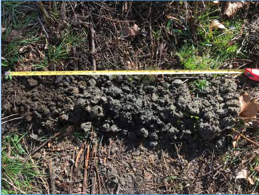
1. Soil Meets A5- Stratified Layers, A12-Thick Dark Surface, and F6-Redox Dark Surface (Profile # 102).
