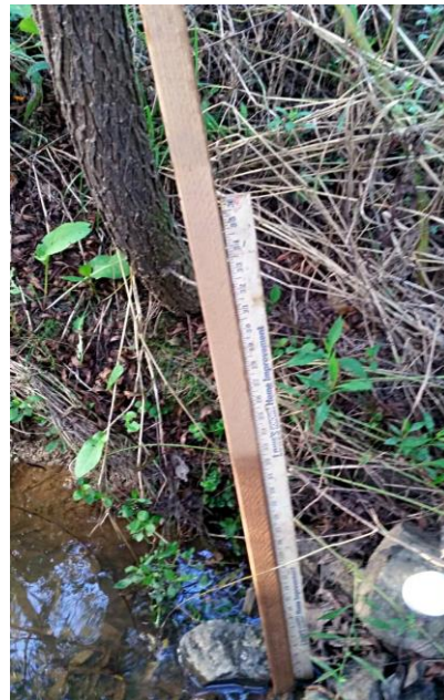
Downstream Crest Stage Gauge, September 2017
