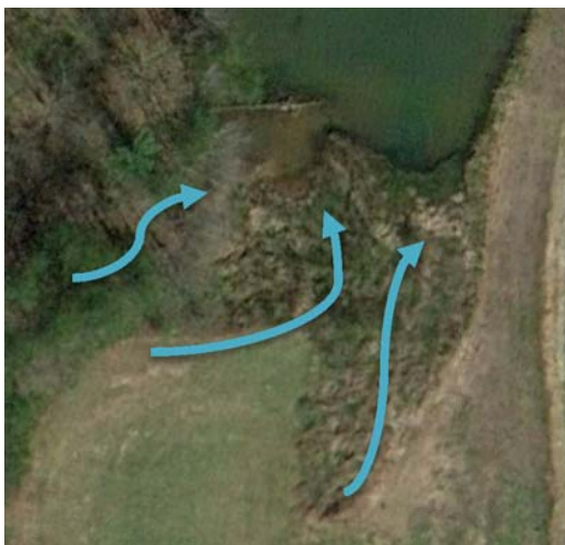
Multiple Channel Threads at Head of Pond 2 as a Result of Loss of Sediment Transport
