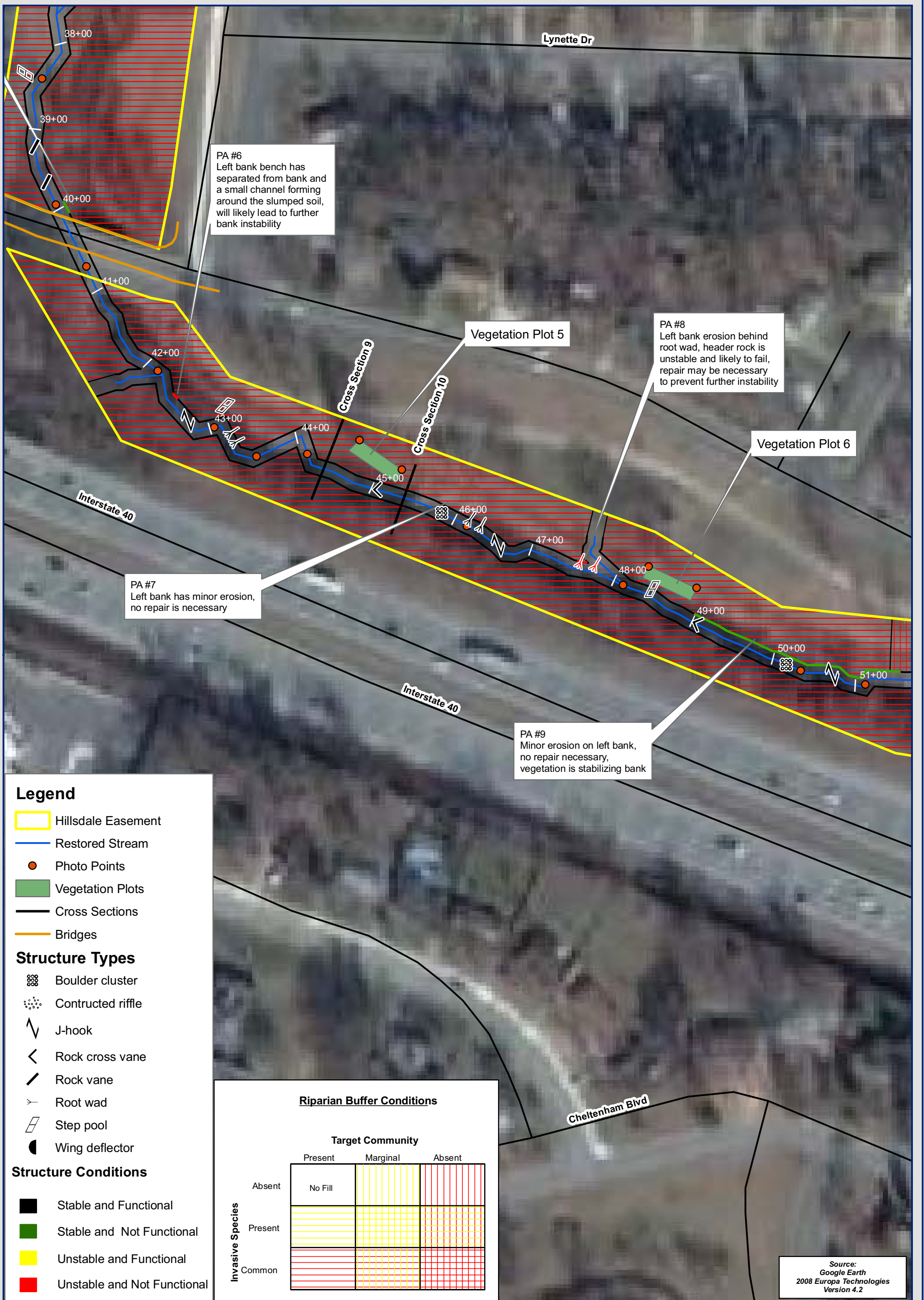
Figure 2 Hillsdale Park Current Condition Plan View (c) Year 5 Monitoring July 2008
