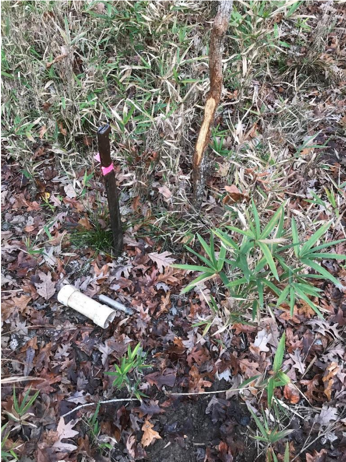
Reference well found damaged. Appears to have been done by deer.
