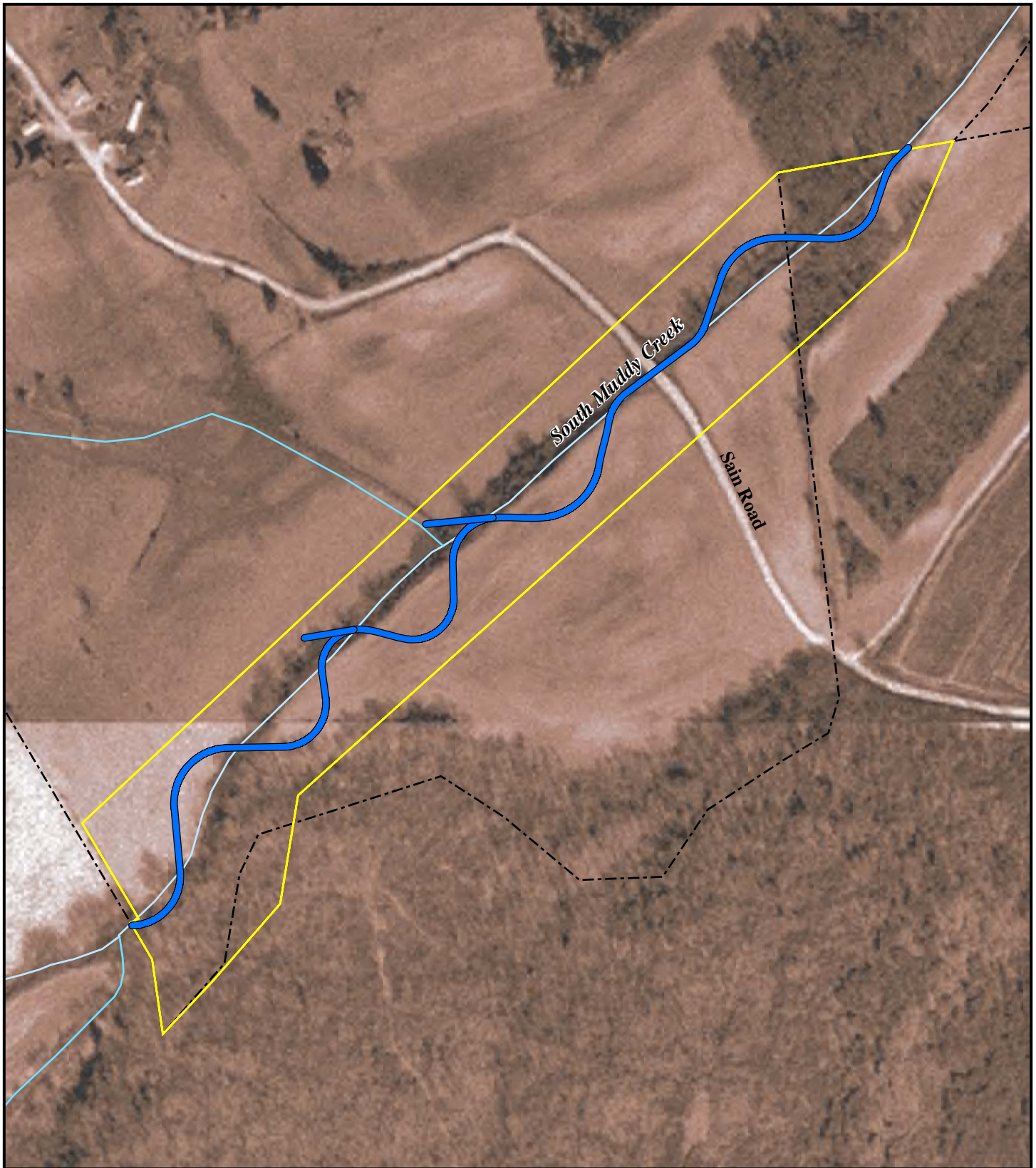
Figure 7.1: South Muddy Creek Proposed Restoration Design South Muddy Creek Stream Restoration Project EEP Project D07032S McDowell County, NC
