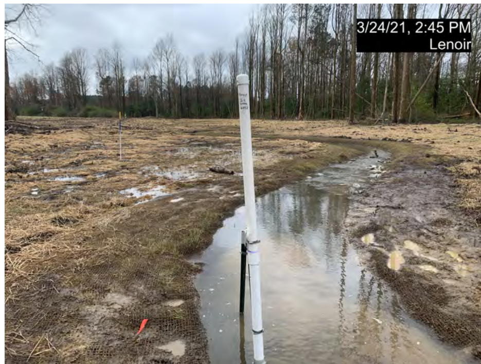
Crest Gauge (CG-1, Pressure Transducer) – MS3
