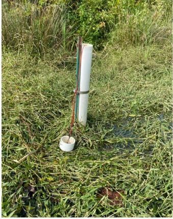
Photo 1: Logger dislodged at monitoring well 10, on the multi-thread channel Reach 5.
