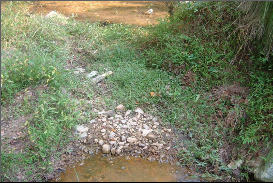
SP5 – Bed aggradation and weedy growth in channel near confluence of UT to Bushy Branch and Bushy Branch. Photo taken near station 03+40. 10/5/06 - MY 02
