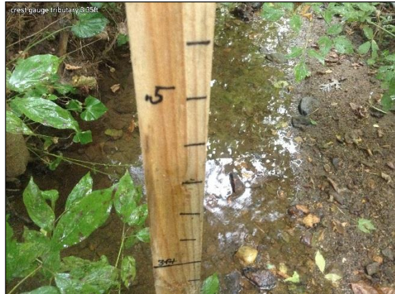
Crest gauge, UT. Cork at 3.35ft. September 29, 2014
