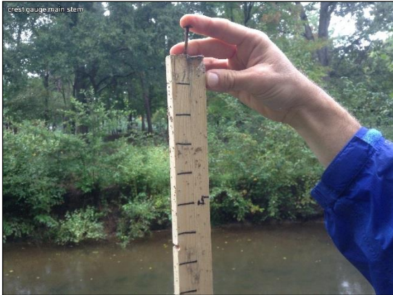
Crest gauge, main stem. Cork overtopped gauge. September 29, 2014
