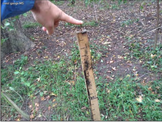
Crest gauge, main stem. Cork overtopped gauge. October 5, 2016
