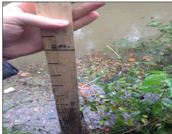
Crest gauge, main stem. Cork at 2.2 ft. September 25, 2015
