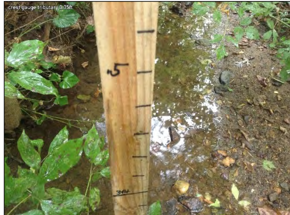
Crest gauge, UT. Cork at 3.35 ft. September 29, 2014
