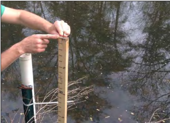
Crest gauge, main stem. Cork overtopped gauge. April 10, 2015
