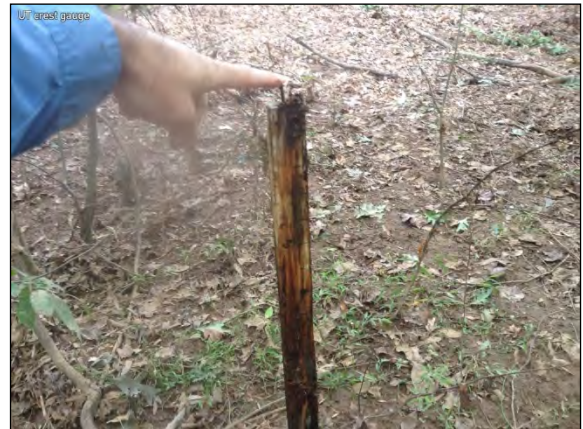
Crest gauge, UT. Cork overtopped gauge. October 5, 2016
