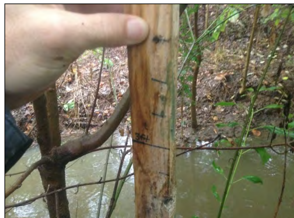
Crest gauge, main stem. Cork at 3.3 ft. September 25, 2015
