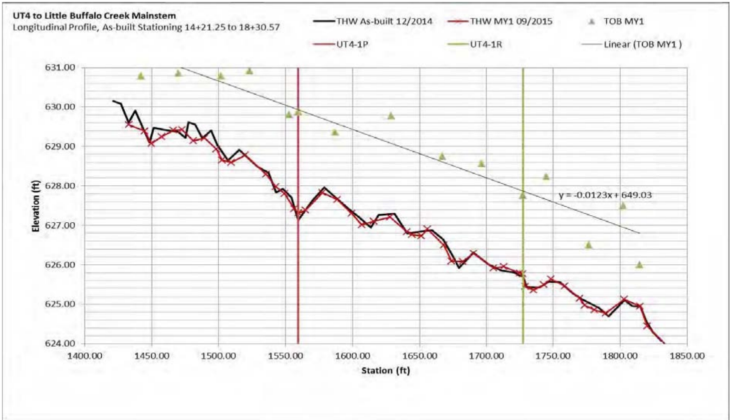
Figure 3i – Longitudinal Profile for UT4 to Mainstem
