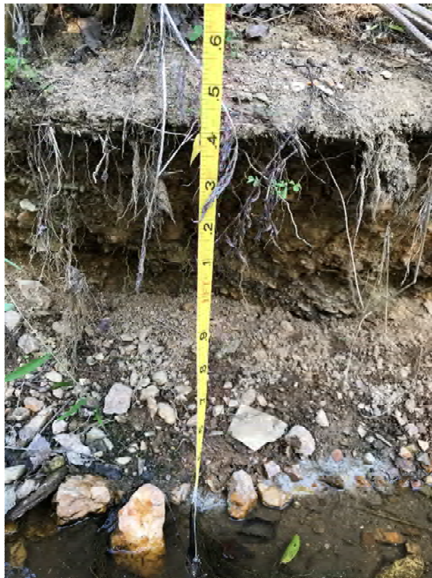
Undercut along the left interior channel bank in restoration area of reach 3
