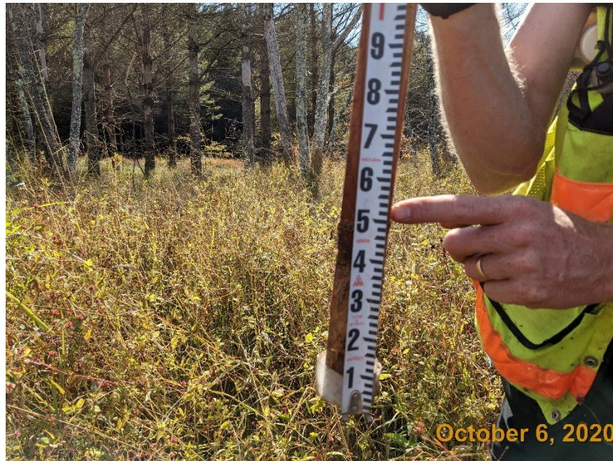
3. Crest gage corklines, LPCII Trib B.
