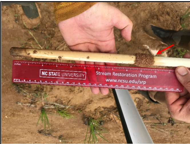
Manual crest gauge on upper R1 reading 0.81 ft (photo: 6/19/19)
