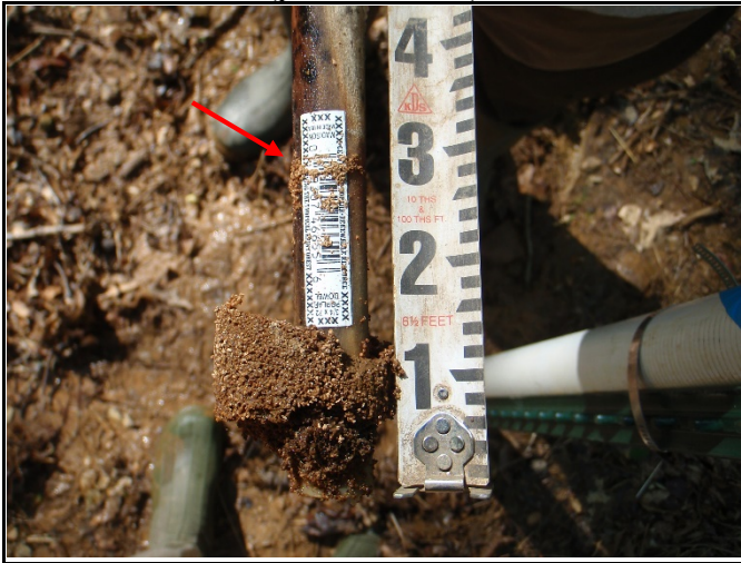
Manual crest gauge on upper R3 reading 0.30 ft (photo: 4/18/19)
