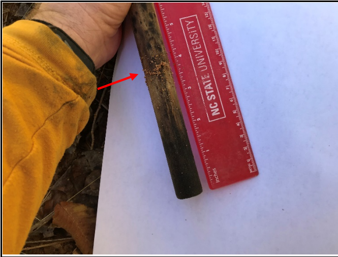
Manual crest gauge on upper R3 reading 0.29 ft (photo: 6/19/19)
