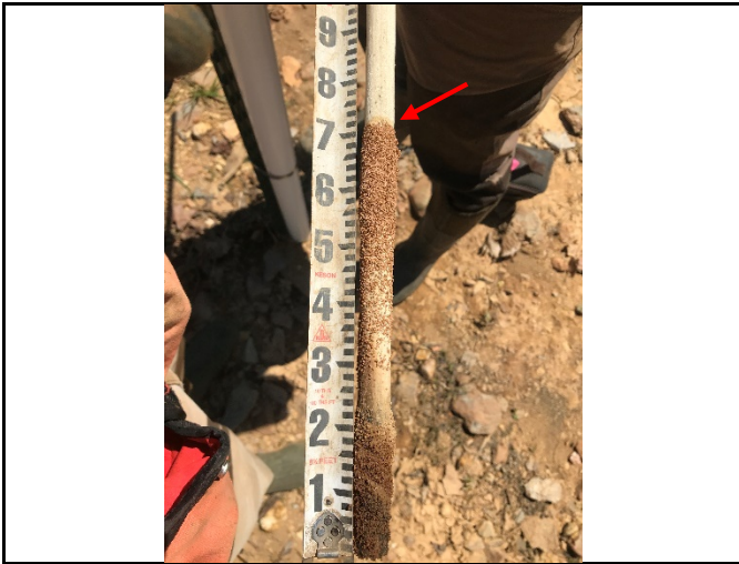
Manual crest gauge on upper R1 reading 0.71 ft (photo: 4/18/19)
