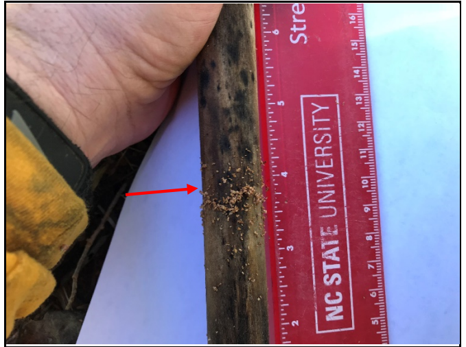
Manual crest gauge on upper R3 reading 0.29 ft (photo: 6/19/19)
