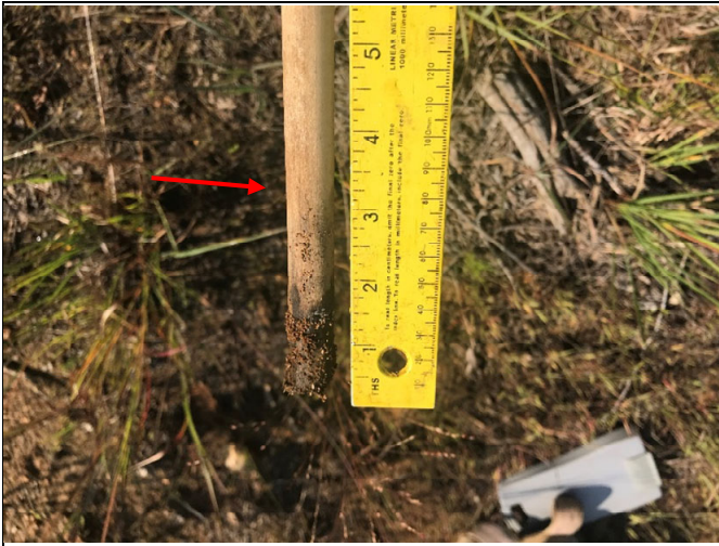
Manual crest gauge reading of 0.23 ft on upper R1 (photo from 5/8/20, storm on 3/25/20)
