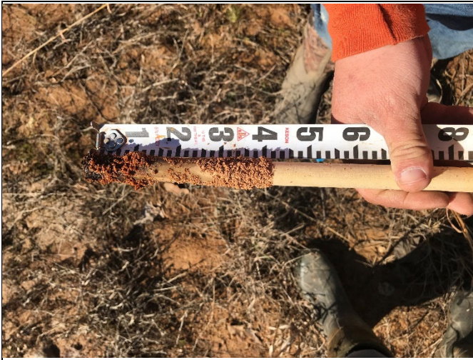
Manual crest gauge reading of 0.41 ft on upper R1 (photo from 2/27/20, storm on 2/27/20)
