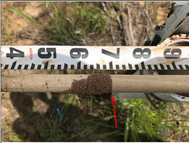
Close-up of manual crest gauge reading of 0.69 ft on upper R1 (photo from 7/10/20, storm on 5/20/20)
