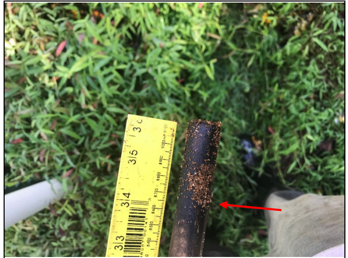
Manual crest gauge reading of 0.16 ft on upper R3 (photo from 7/10/20, storm on 5/20/20)
