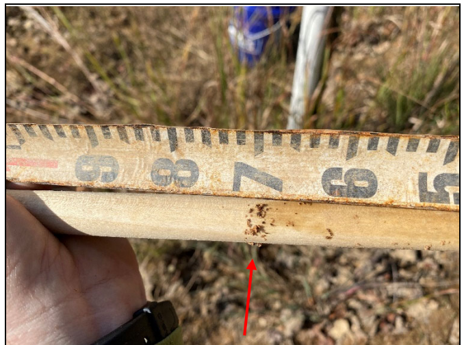
Close-up of manual crest gauge reading of 0.71 ft on upper R1 (photo from 10/14/20, storm [Hurricane Delta] on 10/11/20)
