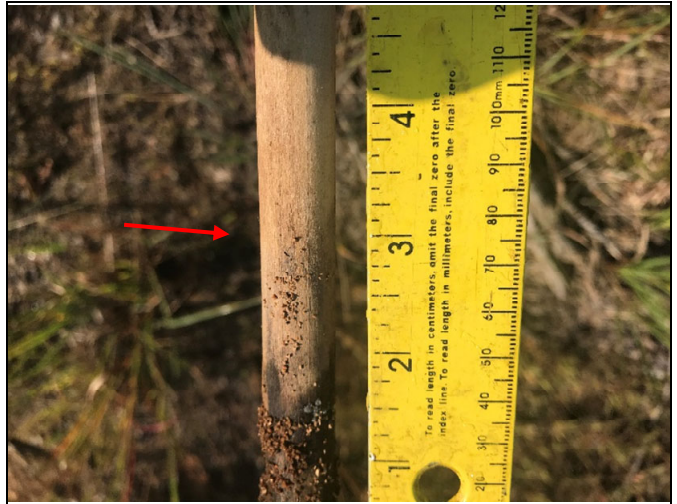
Close-up of manual crest gauge reading of 0.23 ft on upper R1 floodplain (photo 5/8/20 for storm on 3/25/20)
