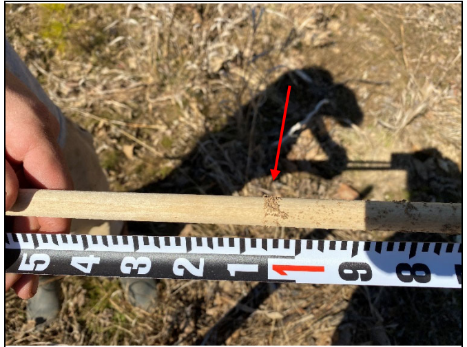
Close-up of manual crest gauge reading of 1.01 ft on upper R1 (photo from 3/11/21, storm on 2/16/21)
