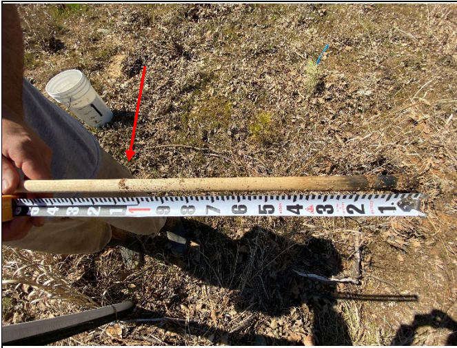
Manual crest gauge reading of 1.01 ft on upper R1 (photo from 3/11/21, storm on 2/16/21)
