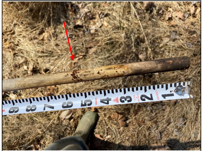
Manual crest gauge reading of 0.56 ft on upper R3 (photo from 3/11/21, storm on 2/16/21)
