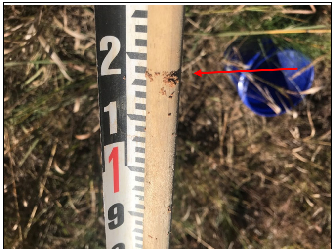
Close-up of manual crest gauge reading of 1.17 ft on upper R1 (photo from 10/20/21, storm from 7/19/21)
