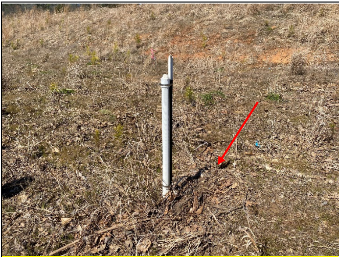
Debris jams around base of crest gauge on upper R1 (photo from 3/11/21)
