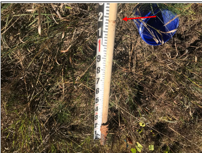
Manual crest gauge reading of 1.17 ft on upper R1 (photo from 10/20/21, storm from 7/19/21)
