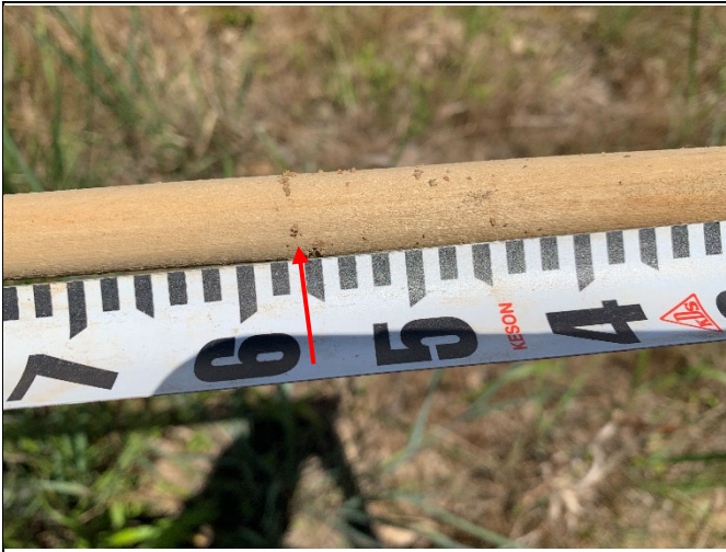
Manual crest gauge reading of 0.57 ft on upper R1 (photo from 6/24/21, storm on 4/9/21)
