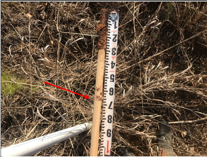
Manual crest gauge reading of 0.67 ft on upper R1 (photo from 3/15/22)
