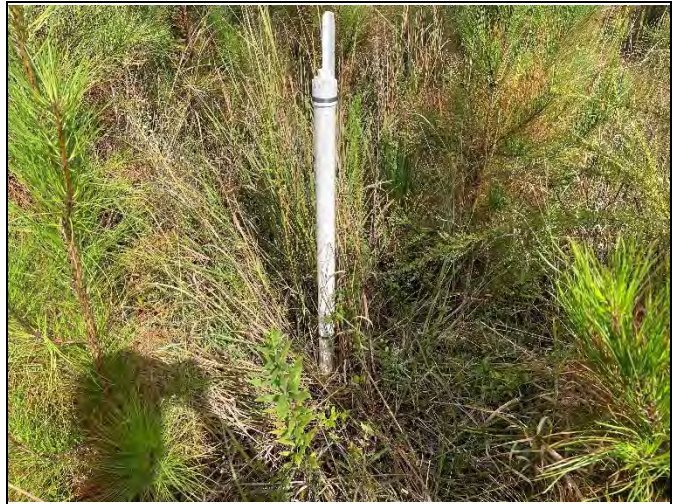
Crest Gauge 2 (cork gauge) on upper R1 floodplain
