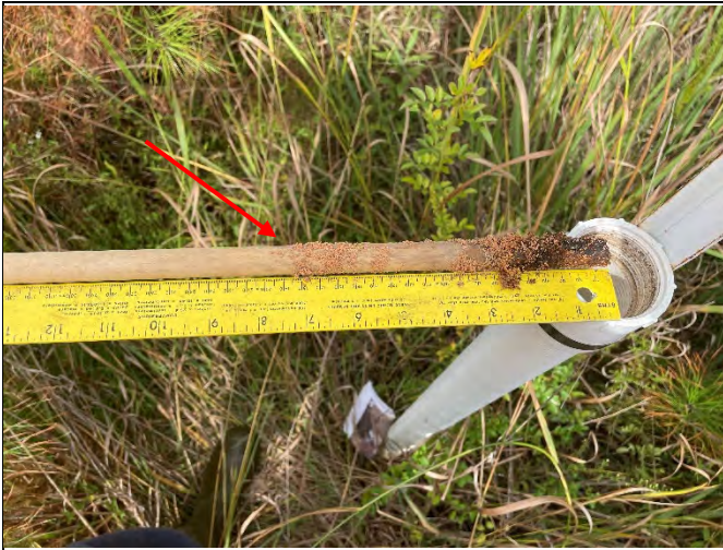
Manual crest gauge reading of 0.59 ft on upper R1 (photo from 8/5/23)
