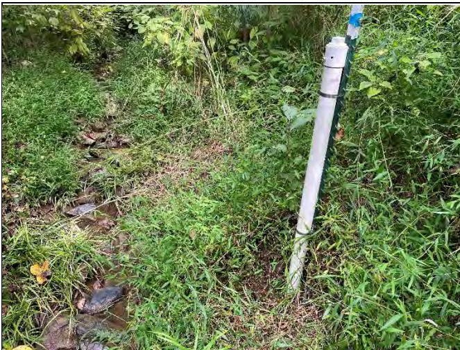
Crest Gauge 3 (instream gauge) on upper R3
