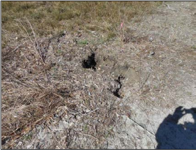
Photo 3. Bank Scour – Station 28+00, Small hole on the floodplain developed from water standing over woody debris of geolift.
