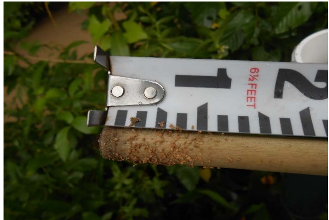
Crest Gauge reading taken on 8/17/16 shows minimal water level rise between 3/18/16 and 8/17/16.
