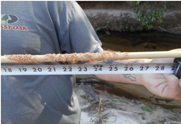
Crest Gauge reading taken on 3/18/16 shows highest water level recorded during high water events that occurred during December 2015 and January 2016.
