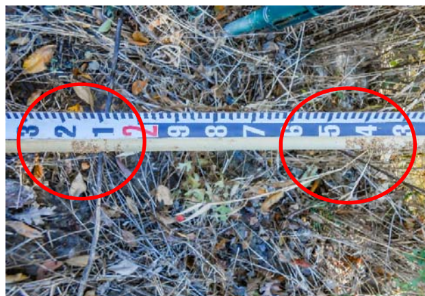
Crest Gauge reading taken on 10/26/2017 shows two distinct high flow events, the lower of which likely occurred on 10/23/2017.
