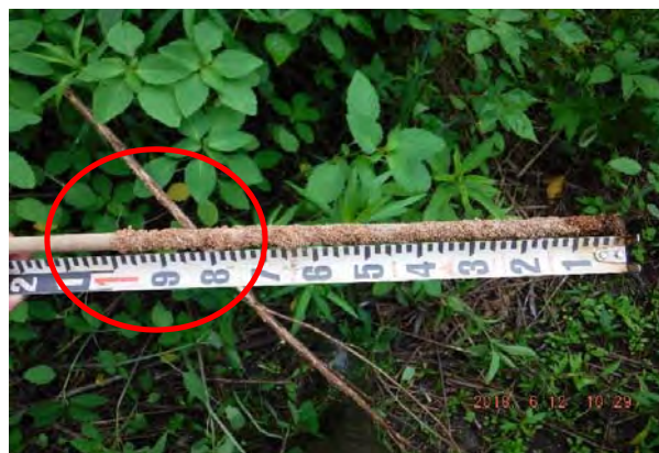
Crest Gauge reading taken on 6/12/2018 shows a distinct high flow event at 11.88 inches on the crest gauge.
