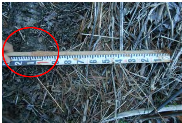
Crest Gauge reading taken on 3/16/2018 shows a distinct high flow event at 12.84 inches on the crest gauge.
