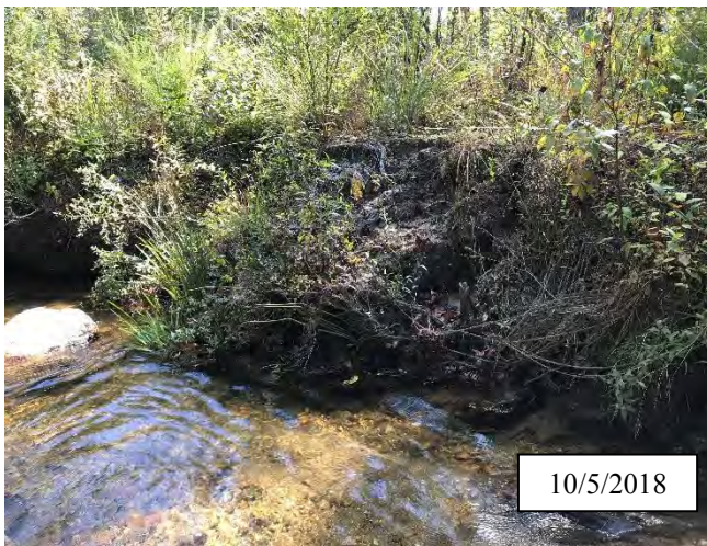
Photo 9. CPA 2-3 – Station 4+60, bank scour area has vegetated but is still eroding. Will be monitored in MY5.
