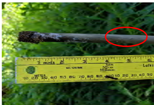
Crest gauge reading taken on 8/8/19 shows a distinct high flow event at 5.2 inches.
