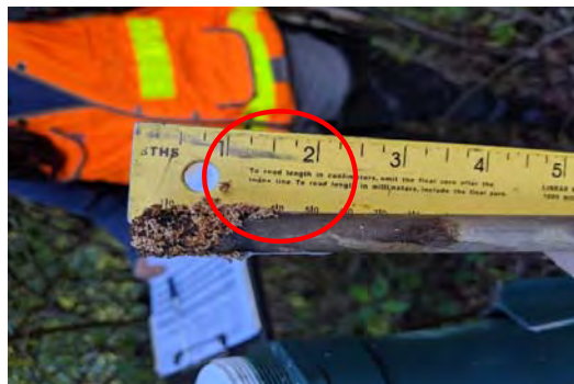
Crest gauge reading taken on 10/23/19 shows a high flow event at 1.5 inches.
