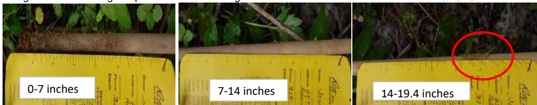
Crest Gauge reading taken on 5/7/2019 shows a distinct high flow event at 19.4 inches. Reading was taken with three consecutive measurements.
