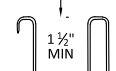
ALTERNATE TYPES OF STAPLES USE ONE #9 STAPLE OR TWO #16 STAPLES AT EACH POINT OF ATTACHMENT.
