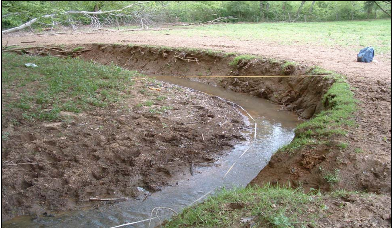
Photograph 37 – Downstream view of Cross-section 4, located on meander with bed morphology that has been significantly disturbed. Channel flow has both run and pool characteristics.
