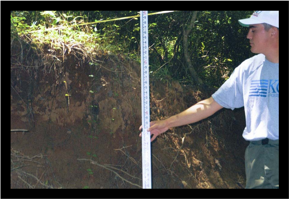
Photo 7: High BEHI scores are common in the upper portion of the project reach.
