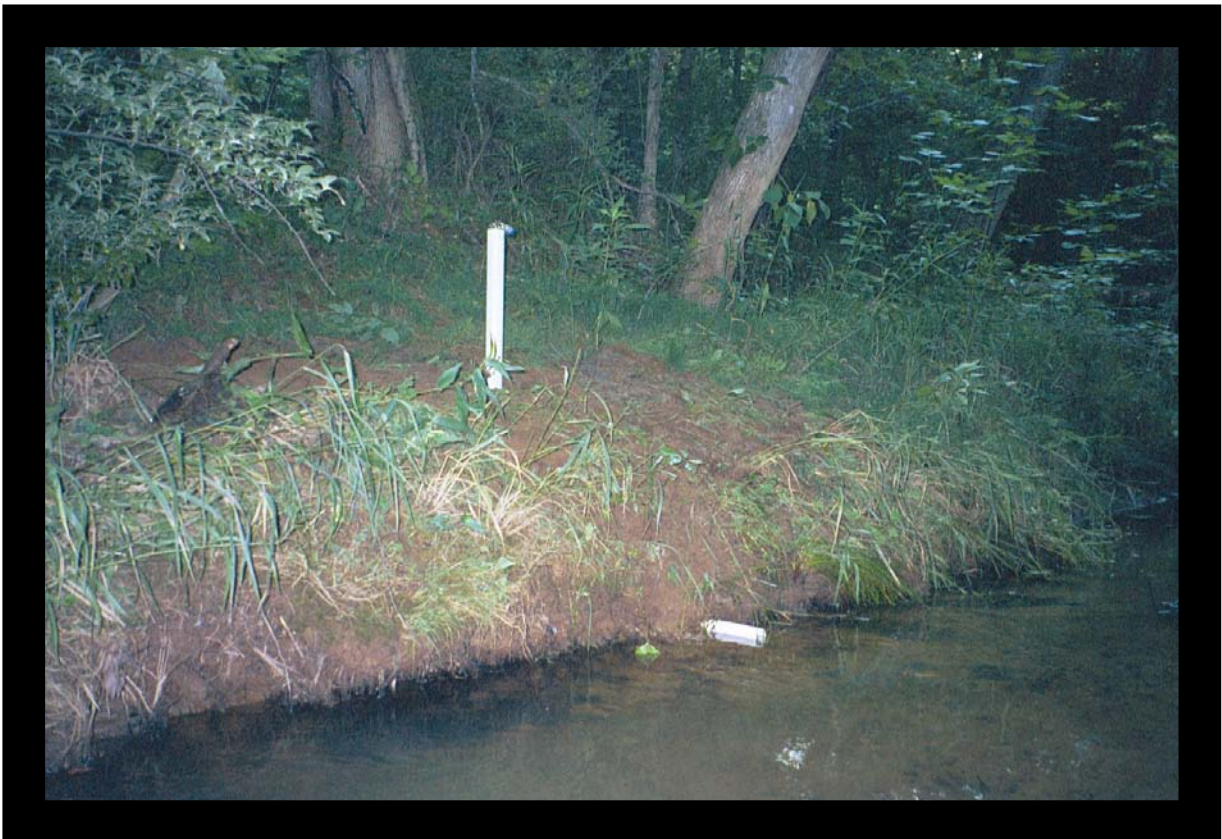
Photo 14: Water level-logging instrument installed at cross section #3 to gauge discharges in McIntyre Creek.
