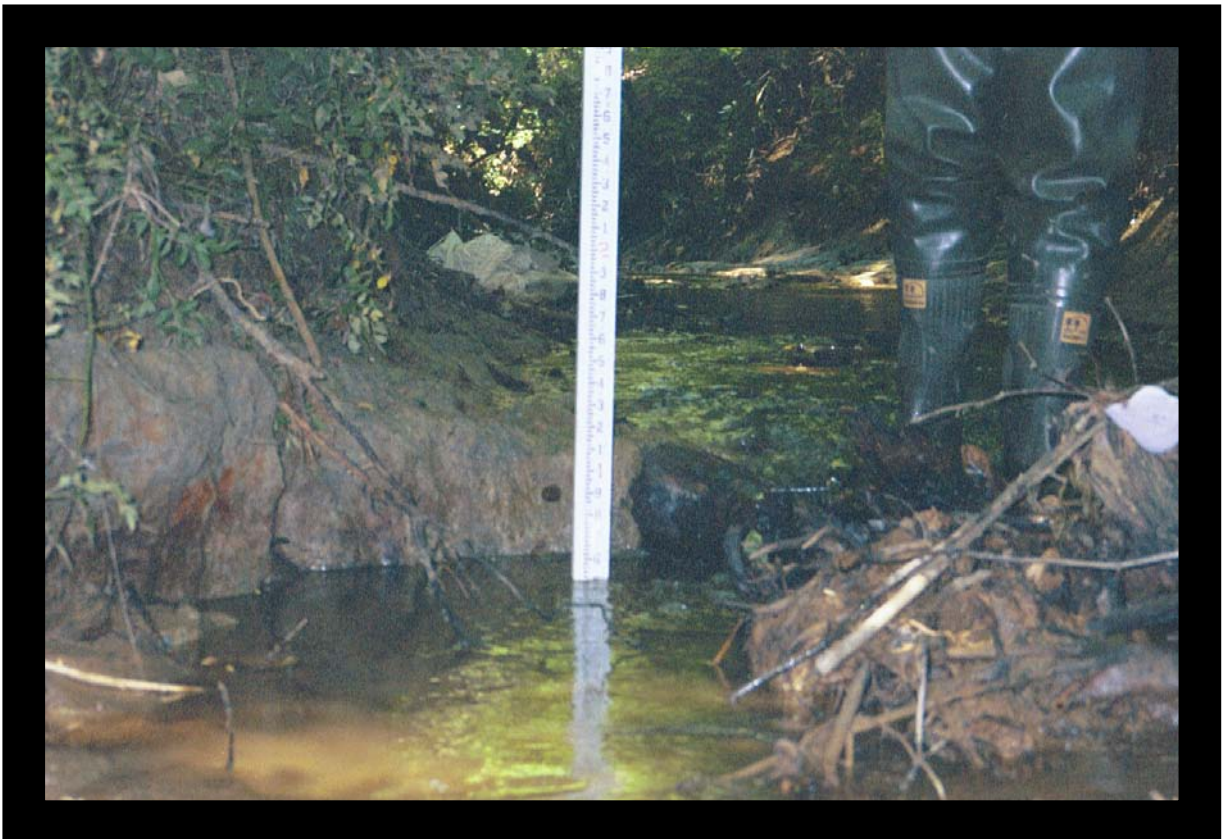
Photo 4: Small knickpoint (approximately 14" high) indicating limit of headward erosion in this reach. (Approximate location = Station 14+00.)
