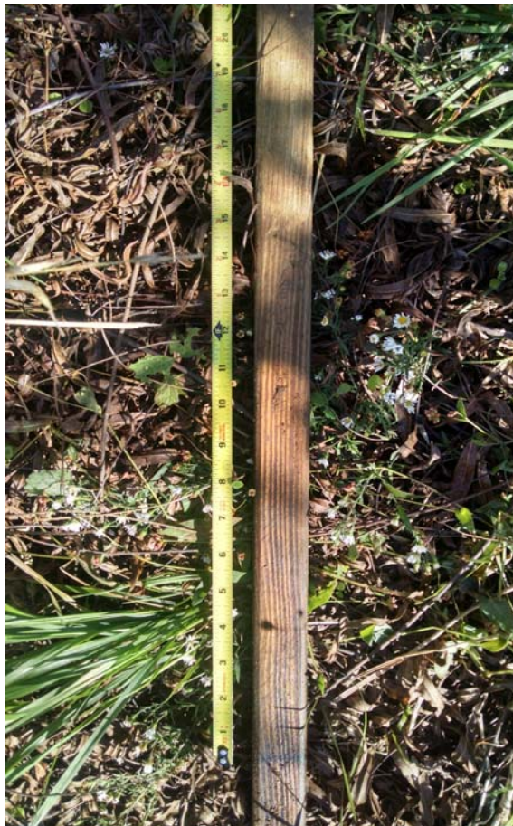
SP1: Crest Gauge Reading
