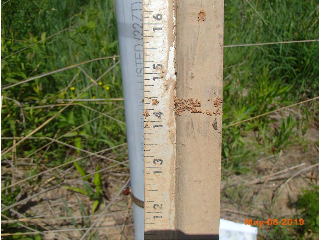
Photo #3 – South Muddy Creek Crest Gauge at 14 inches
