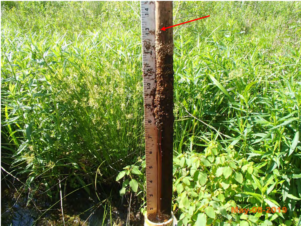
Photo #2 – Sprouse Branch Crest Gauge at 13 inches (recorded bankfull is 9”)
