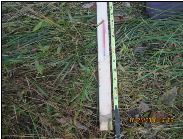
Photo 2 – Crest Gauge on Silage Tributary Reach 2 Station 25+50
