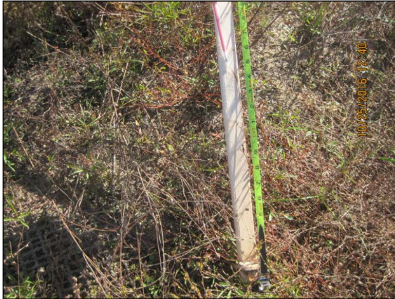
Photo 1 - Crest Gauge on Moore's Fork Reach 2 Station 30+00
