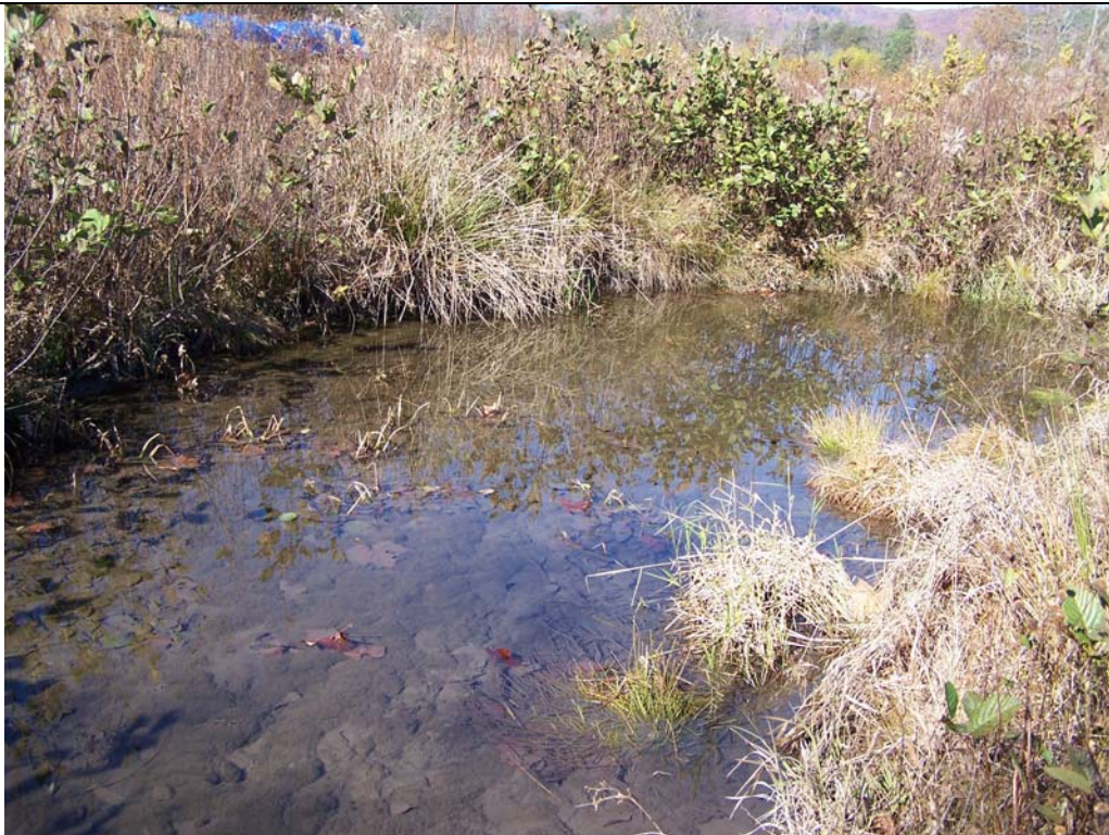
SPA 5 UT1 Sta. 2002+40 – Reduced pool depth due to aggradation November 11, 2010
