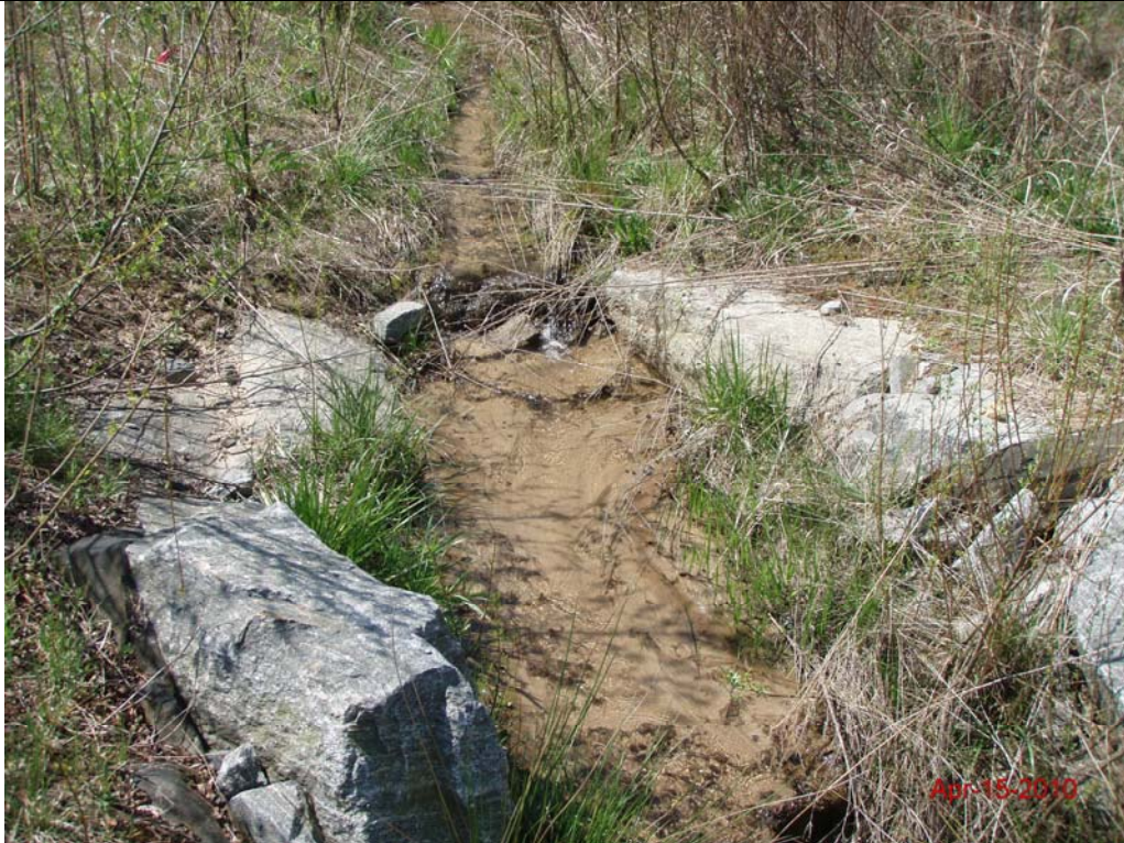
SPA 8 UT2 Sta. 3000+50 – Reduced pool depth and riffle fining due to aggradation April 15, 2010
