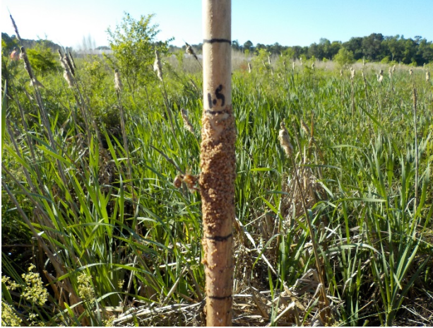
Crest Gauge 1 Reading 1.5' (4/24/2017)
