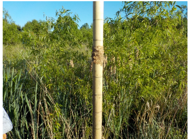
Crest Gauge 4 Reading 2.05' (4/24/2017)
