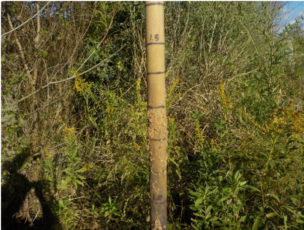
Crest Gauge 2 Reading 1.3' (8/24/2017)
