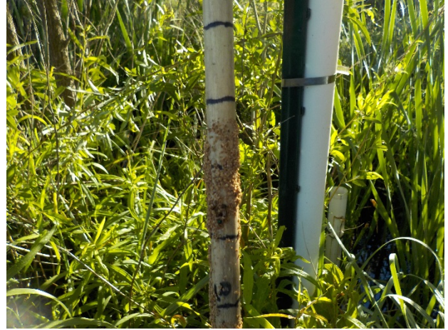
Crest Gauge 3 Reading 1.27' (4/24/2017)
