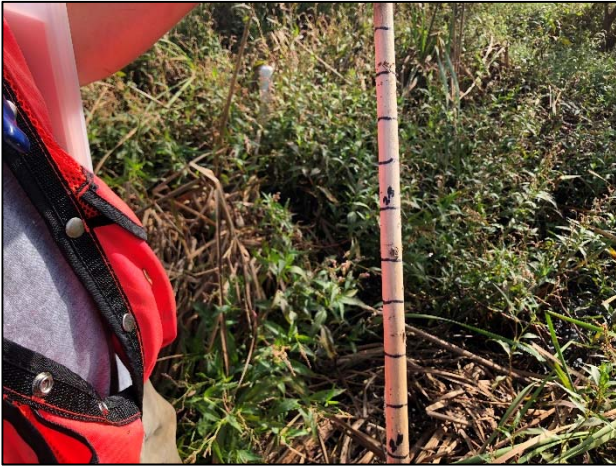
Crest Gauge 1 Reading: 2.82 feet
