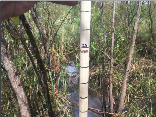
Crest Gauge 3 Reading: 2.48 feet
