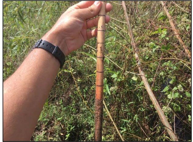
Crest Gauge 2 Reading: 1.4 feet
