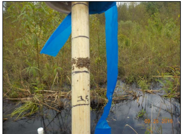
Crest Gauge 4 Reading: 3.65 feet
