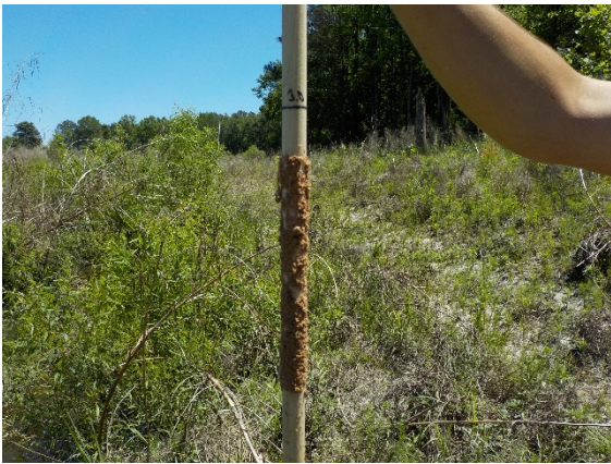
Photo 3. Crest Gauge 4 (Reach 5A – 2.8 ft. – 4/24/17)
