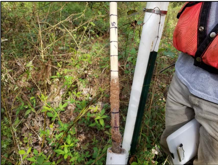
Photo 3. Crest Gauge 3 (Reach 3B – 0.65 – 9/15/2018)
