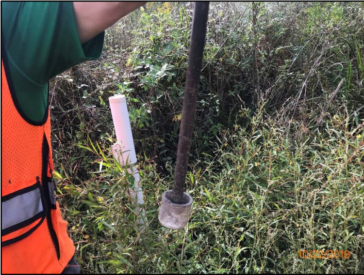
Photo 1. Crest Gauge 2 (Reach 3a – 0.63 ft. – 9/5/2019)
