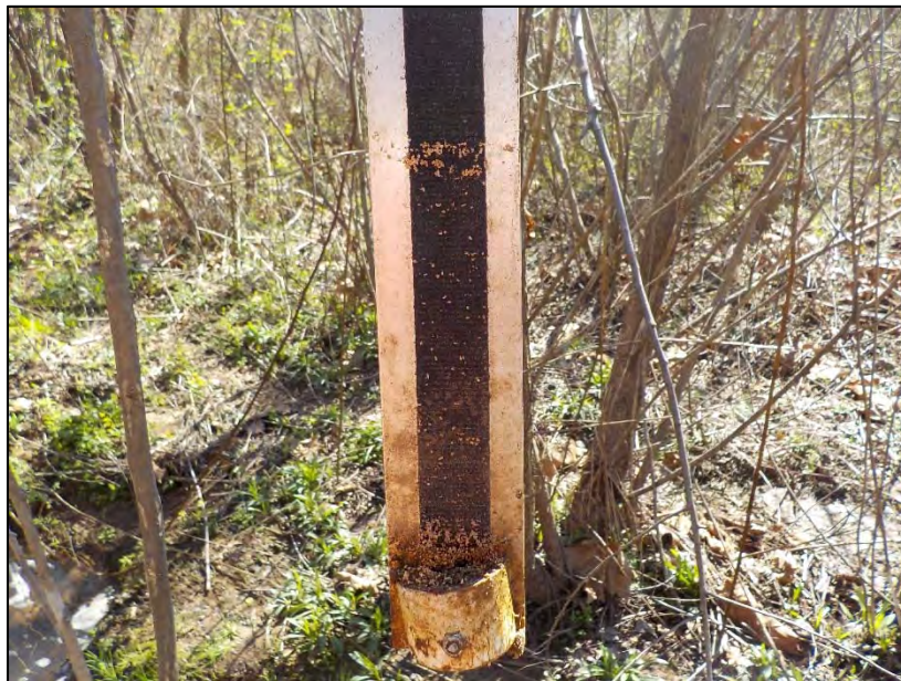
Crest Gauge @ Reach 2 – 0.58 ft above bankfull
