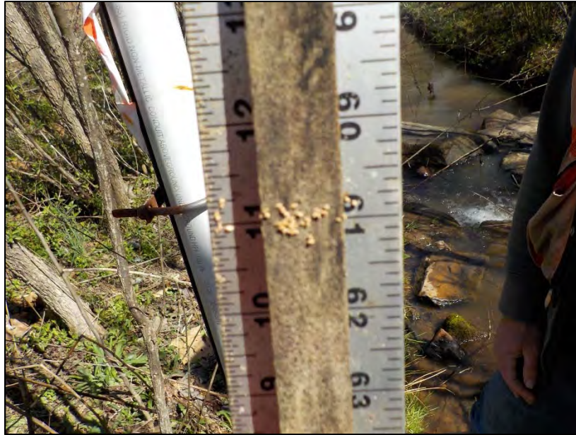
Crest Gauge @ Reach 4 – 0.92 ft above bankfull
