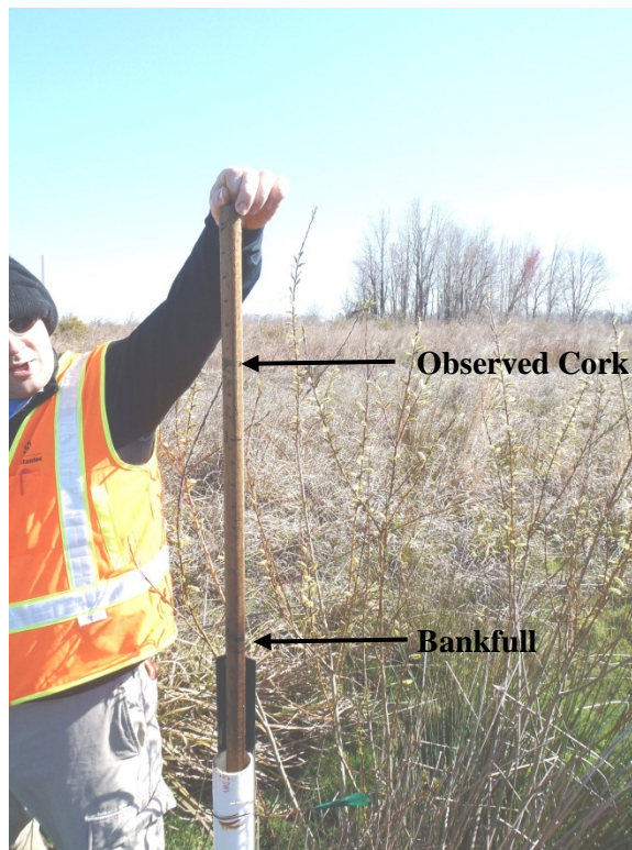
Photo Station S8 – Crest gauge indicating a bankfull event (3/28/2013 Year 3)
