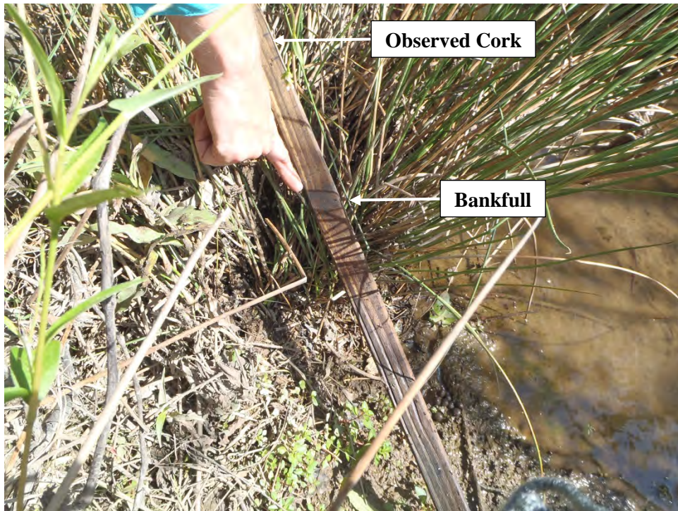
Photo Station S8 – Crest gauge indicating a bankfull event (09/16/2015 Year 5)
