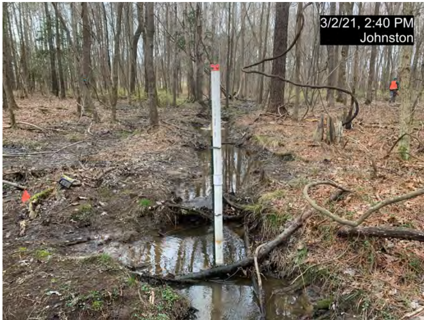
Crest Gauge (CG-2, Pressure Transducer) – R7 lower
