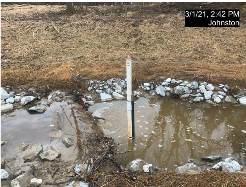
Crest Gauge (CG-1, Pressure Transducer) – R3
